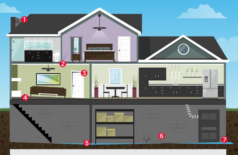
Every home is built on a foundation that supports the building's structure. Residential homes may have a slab, crawl space or basement as part of the foundation. When the foundation is compromised, various problems such as sagging floors, bowed walls and other issues become visible within the home. In many areas, foundation problems begin with the soil underneath and surrounding the house.
